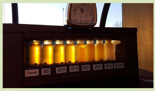
Could purchase internal heating for pump Blend before cold weather approaches Additives should be applied and mixed well
